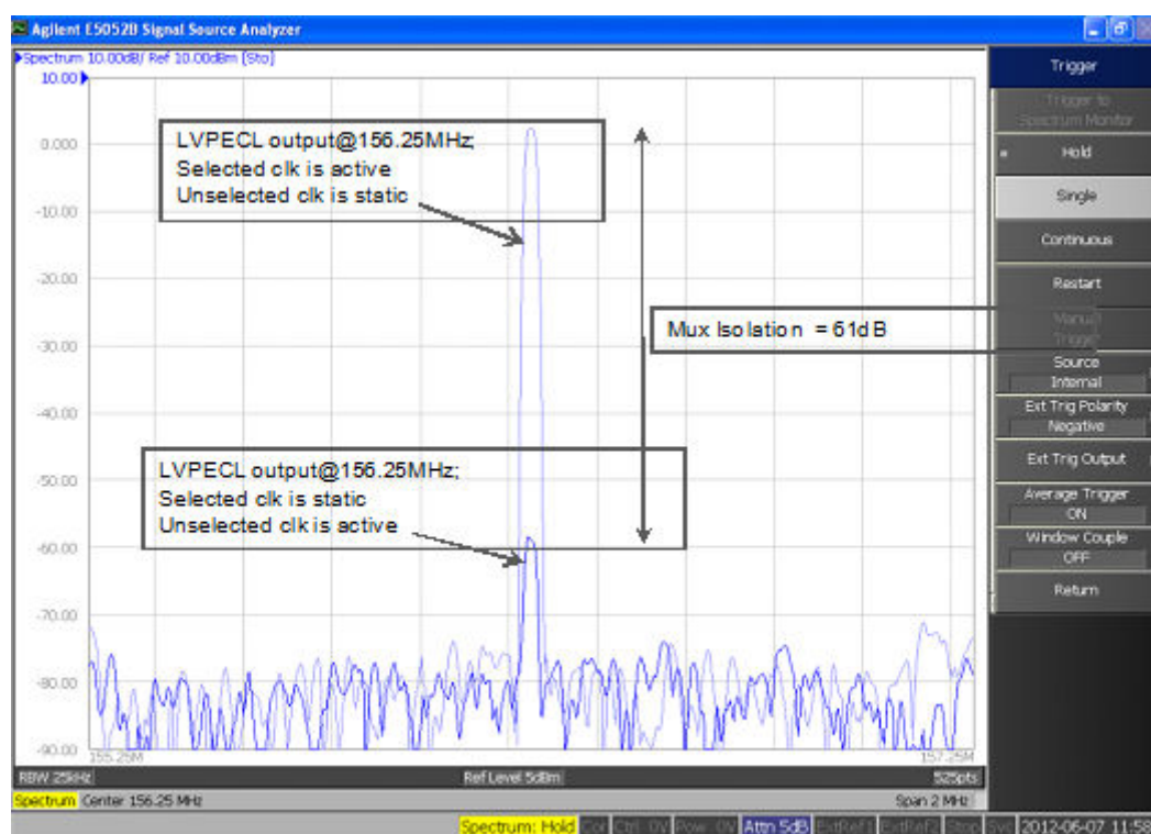
Figure 2.14. Input Mux Noise Isolation (Differential Input Clock, 44-QFN Package)
