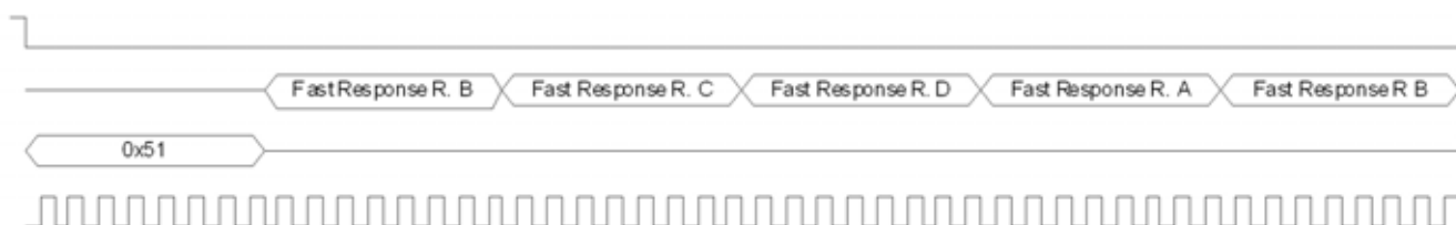
Figure 14. Reading More Fast Response Registers in a Single SPI Transaction
