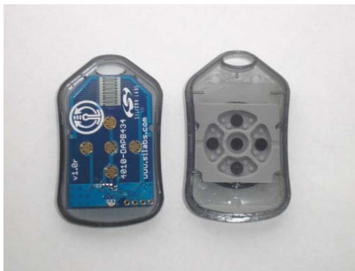
Figure 1. 4010 RKE Universal Key Fob and Plastic Case (P/N 4010-DAPB_434 and MSC-PLPB_1)
