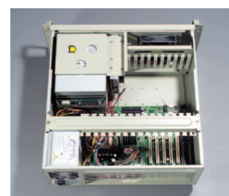
Motherboard can fit in 450 mm (17.7") depth
