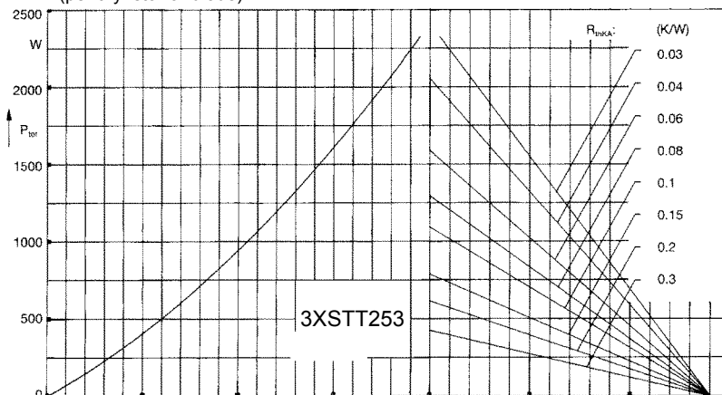
Fig. 5 Three phase rectifier bridge: Power dissipation versus direct output current and ambient temperature
