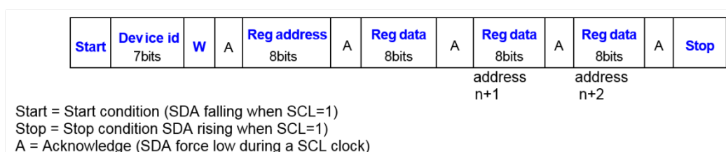
Figure 63. I 2 C write operation
