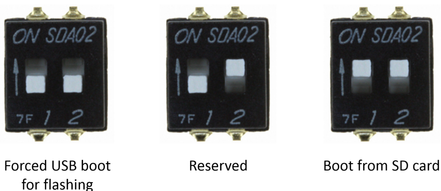
Figure 7. Boot-mode switch SW1
