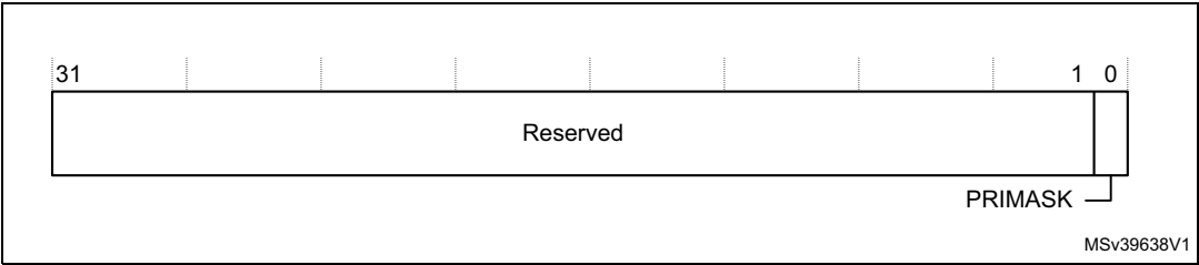
Figure 4. PRIMASK bit assignments:
