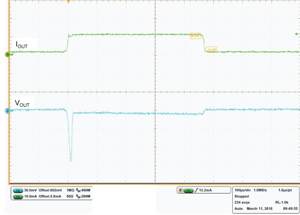
Figure 29. Load transient ( t_{rise} = 5 \mu s )
