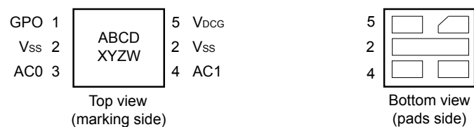
Figure 5. 5-pin package connections - ST25TA02KB-P
