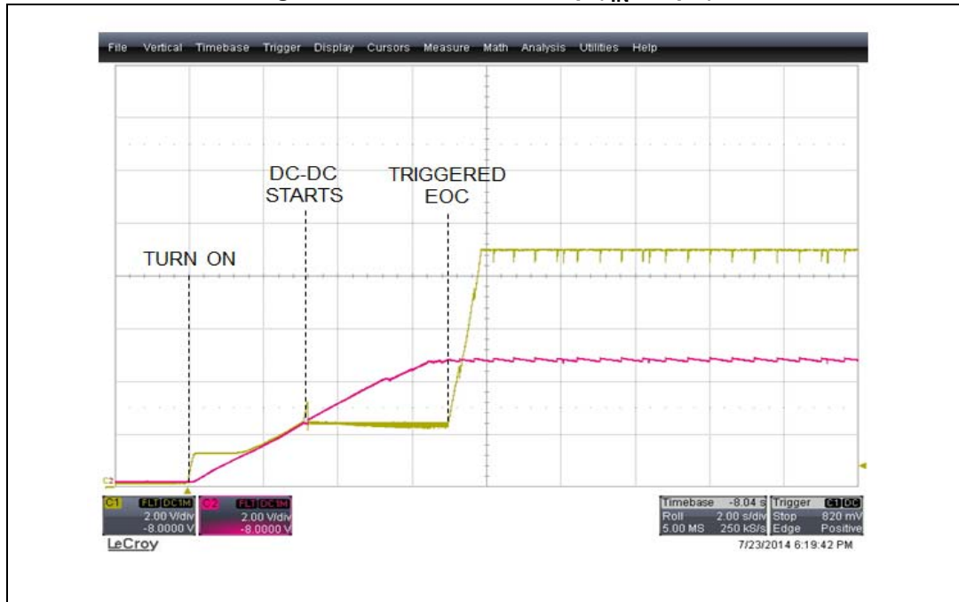
Figure 13. Buck-boost startup ( I_{IN} = 5 \mu A )
