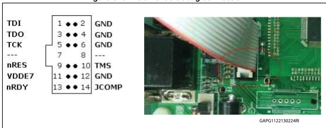
Figure 8. JTAG / Nexus debug connection
