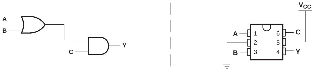
Figure 3. Y = (A + B) \bullet C
