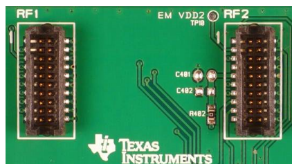
Figure 18. SmartRF06EB EVM Connectors RF1 and RF2
