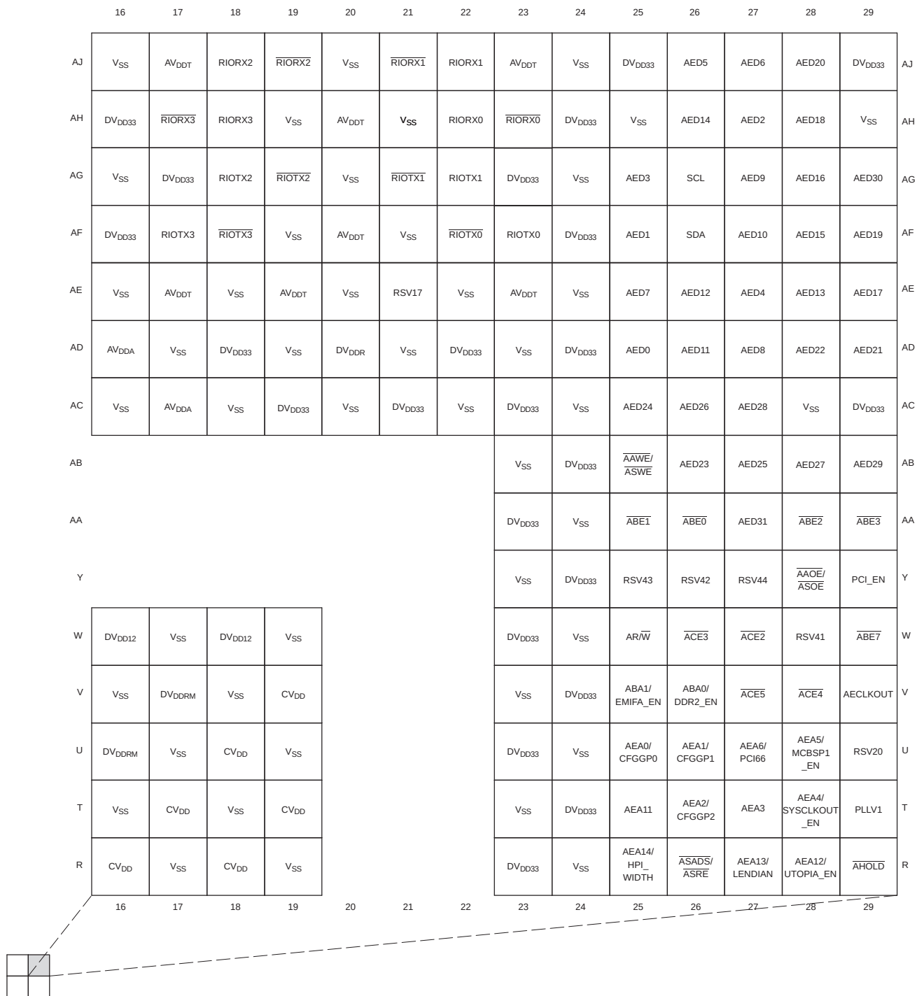
Figure 2-3. C6455 Pin Map (Bottom View) [Quadrant B]
