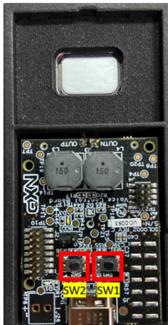
Figure 11. SW1 and SW2 on the SLN-LOCAL-IOT Kit.
