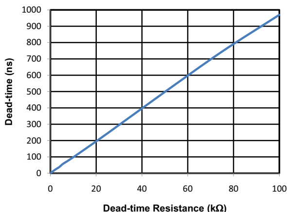
Figure 37. Dead Time vs. Resistance ( R_{DT} )
