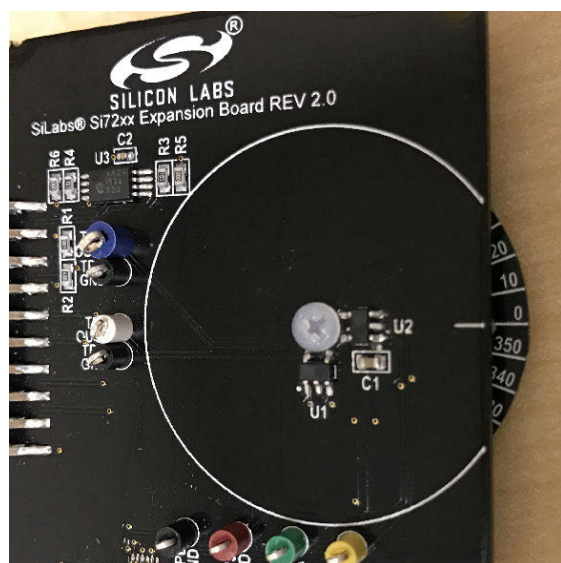
Figure 1.2. Si72xx-EXP Wheel Alignment
