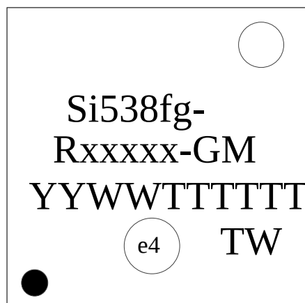
Figure 12.1. Si5381/82 Top Marking
