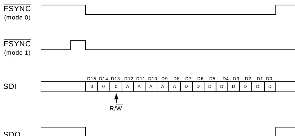
Figure 22. Secondary Communication Data Format—Write Cycle
