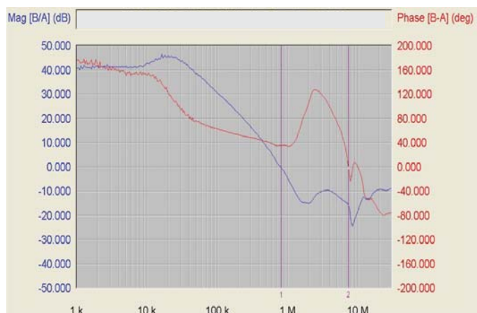
Figure 2 — Gain and Phase Bode Plot F_c = 810\text{KHz} , PM = 36 degree at 1A Source
