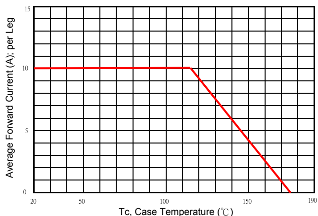
Typical Forward Current Derating Curve
