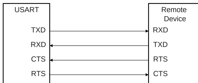
Figure 24-18. Connection with a Remote Device for Hardware Handshaking
