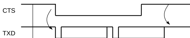
Figure 31-19. Transmitter Behavior when Operating with Hardware Handshaking
