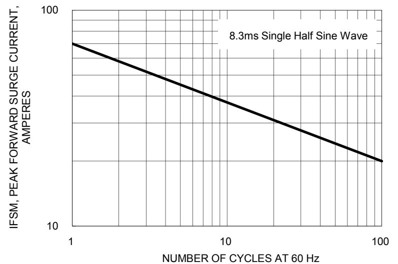
FIG. 4- MAXIMUM NON-REPETITIVE FORWARD SURGE CURRENT UNIDIRECTIONAL ONLY
