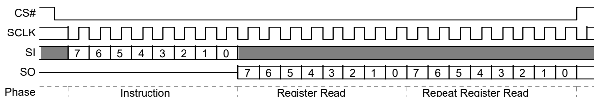
Figure 52. Read Configuration Register (RDCR) Command Sequence
