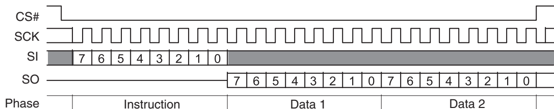
Figure 9. Single Bit Wide I/O Command without Latency
