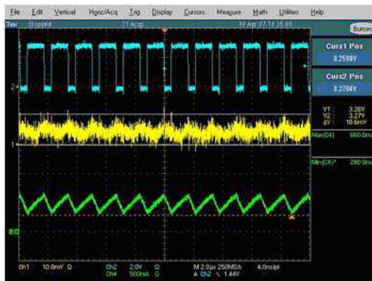
Figure 14. Ceramic 10μF 0603 (X5R) (Good)
