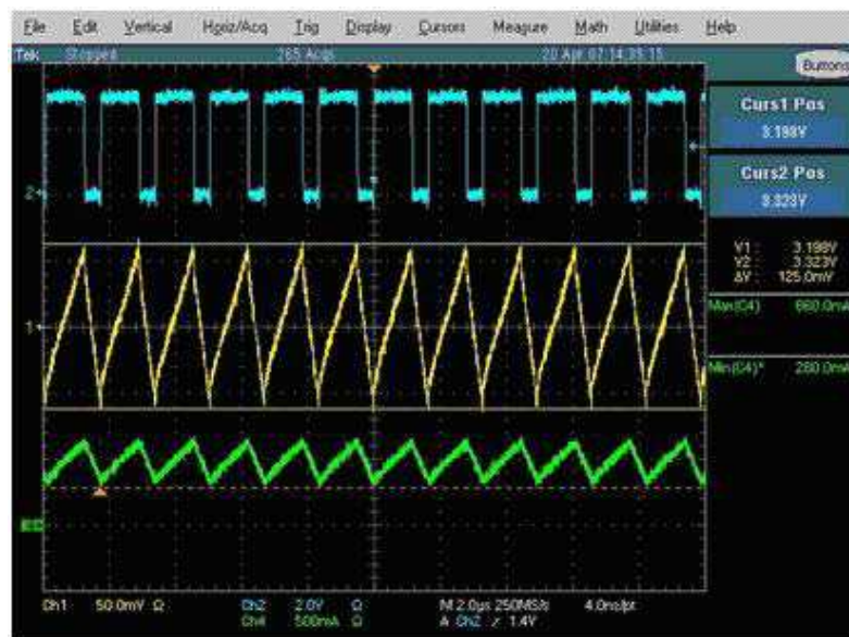
Figure 21. Electrolytic 100 \mu F (Ripple Too High)
