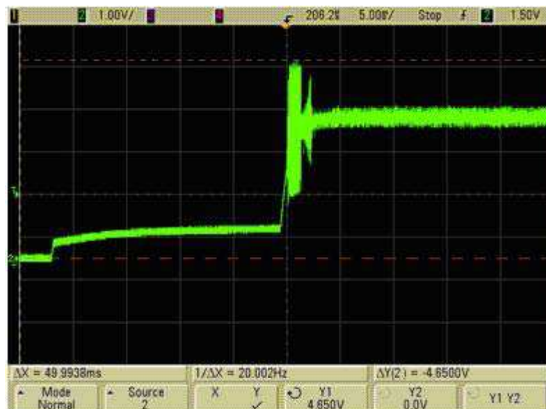
Figure 13. Input Voltage Overshoot >4V (Bad)
