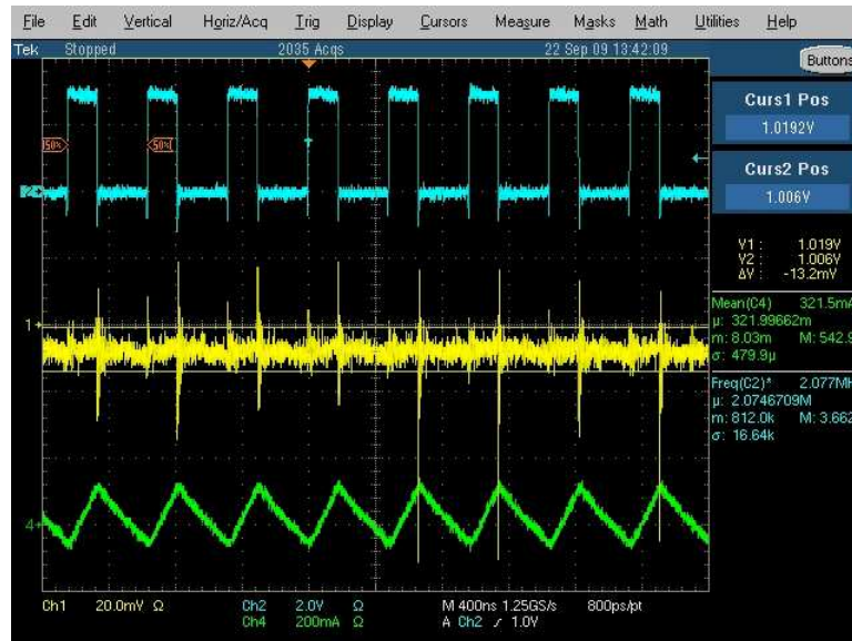
Figure 16. L=GLK2510P-2R2M, C=Ceramic 10 \mu F 0603 X5R YAGEO (Ripple 13.2mV)
