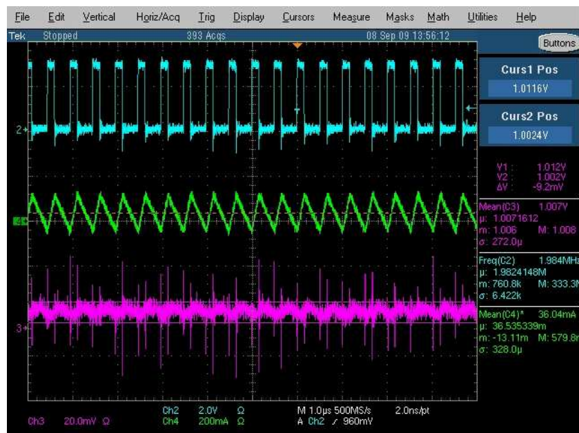
Figure 19. L=GTSD32P-2R2M, C=Ceramic 4.7 \mu F 0805 X5R TDK (Ripple 9.2mV)
