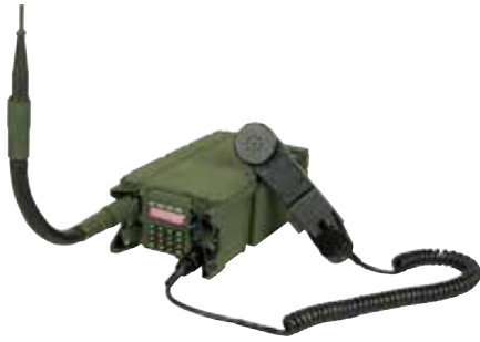
RT-1523 5 W manpack dismount configuration
