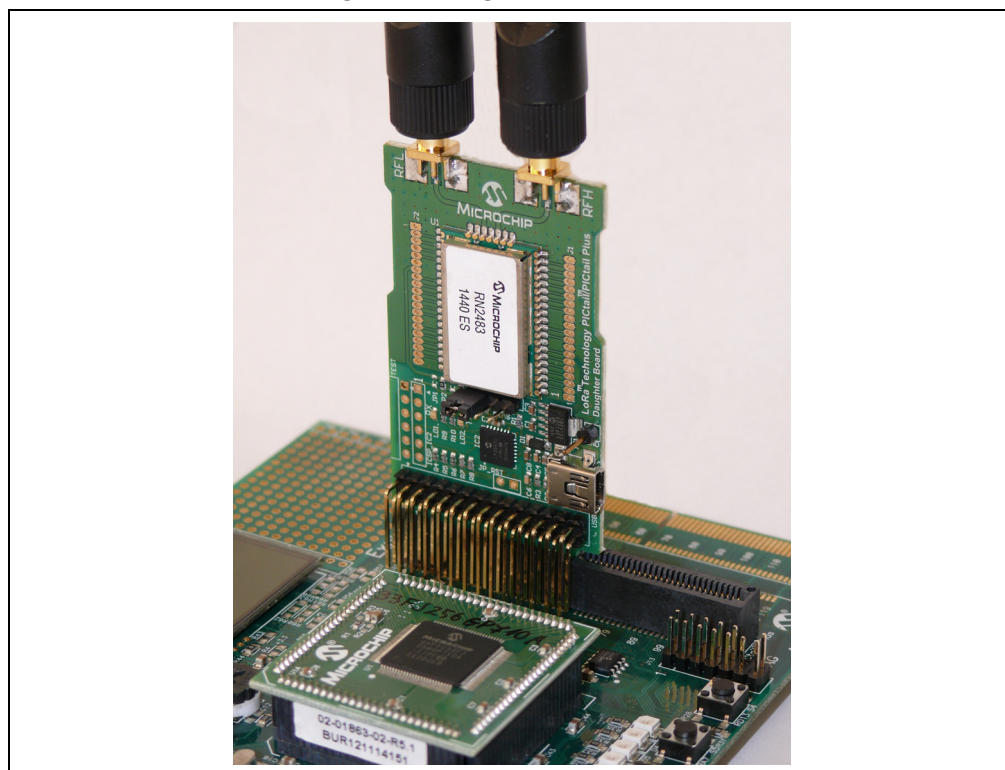
FIGURE 1-2: RN2483 LORA™ TECHNOLOGY PICTail™/PICTail PLUS DAUGHTER BOARD CONNECTED TO EXPLORER 16 DEVELOPMENT BOARD
