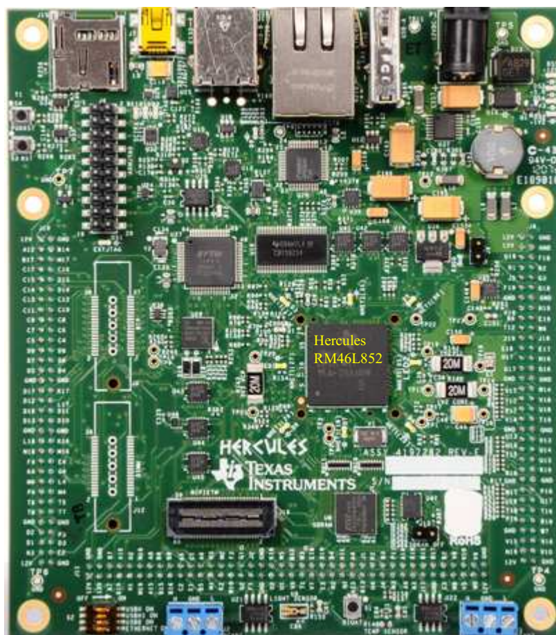
Figure 2-1. RM46 HDK Board, Interfaces Top Side
