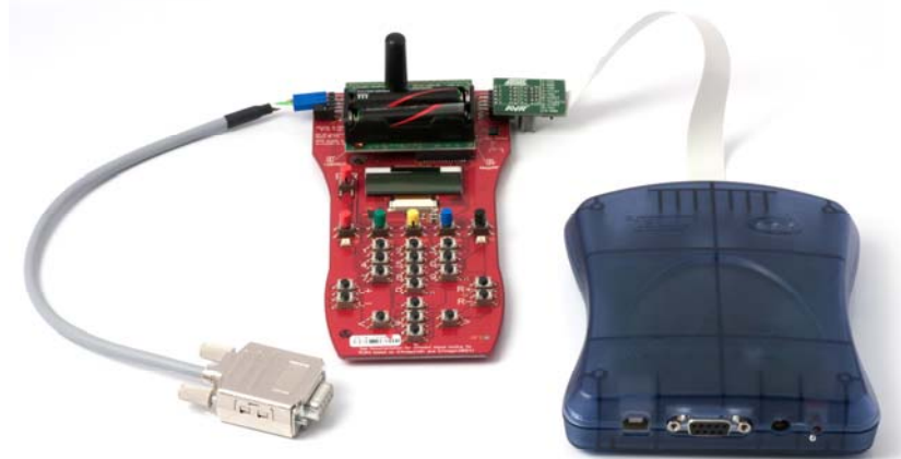
Figure 4-5. KeyRemote with AVR JTAGICE mkII connected.
