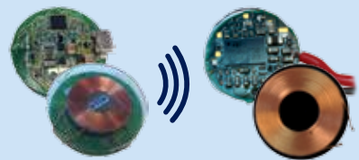
STEVAL-ISB038V1 Wireless charging reference design kit for wearables based on STWBC-WA and STWLC04
