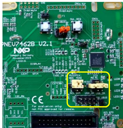
Fig 20. Host Interface selection - SPI
