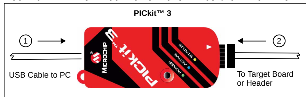
FIGURE 3-1: INSERT COMMUNICATIONS AND USB/POWER CABLES
