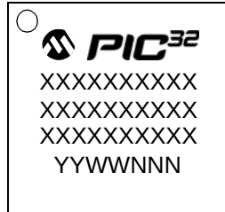
64-Lead QFN (9x9x0.9 mm)
