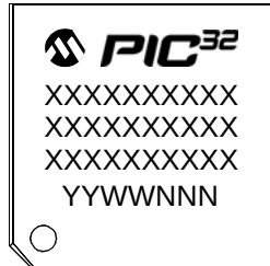
64-Lead TQFP (10x10x1 mm)
