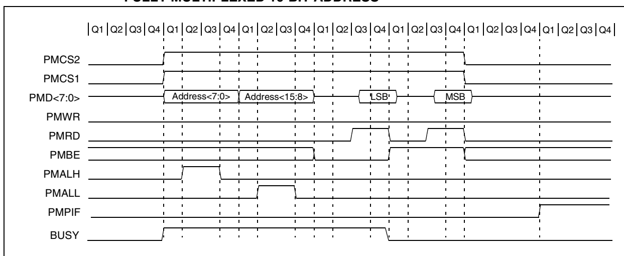
FIGURE 11-25: READ TIMING, 16-BIT MULTIPLEXED DATA, FULLY MULTIPLEXED 16-BIT ADDRESS
