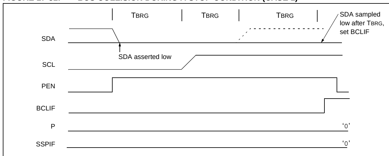
FIGURE 17-31: BUS COLLISION DURING A STOP CONDITION (CASE 1)
