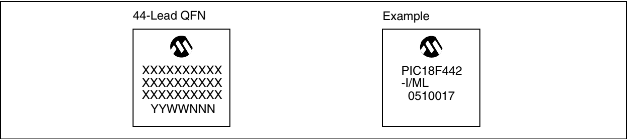
FIGURE 2: PACKAGE MARKING TEMPLATE FOR PIC18F442/452, 44-PIN QFN
