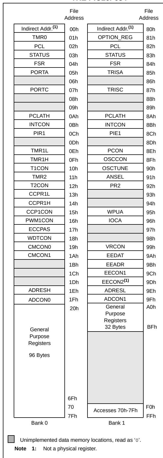
FIGURE 2-2: DATA MEMORY MAP OF THE PIC16F684
