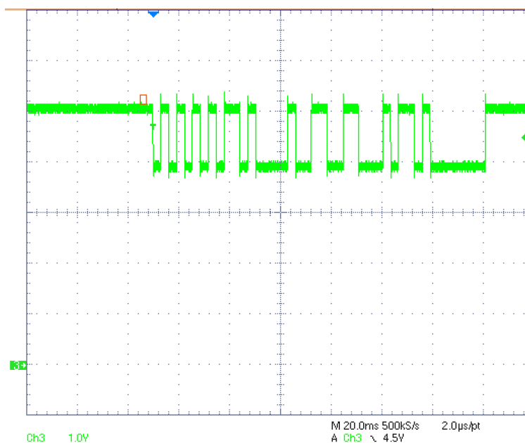
Figure 9. OWI Data at 320 bps; Oscilloscope Probe is Connected at TP20 in the PGAxXXEVM-034
