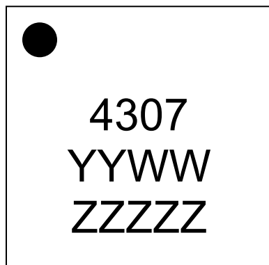
Figure 21. Top Marking Specifications
