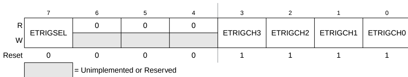
Figure 4-4. ATD Control Register 1 (ATDCTL1)
