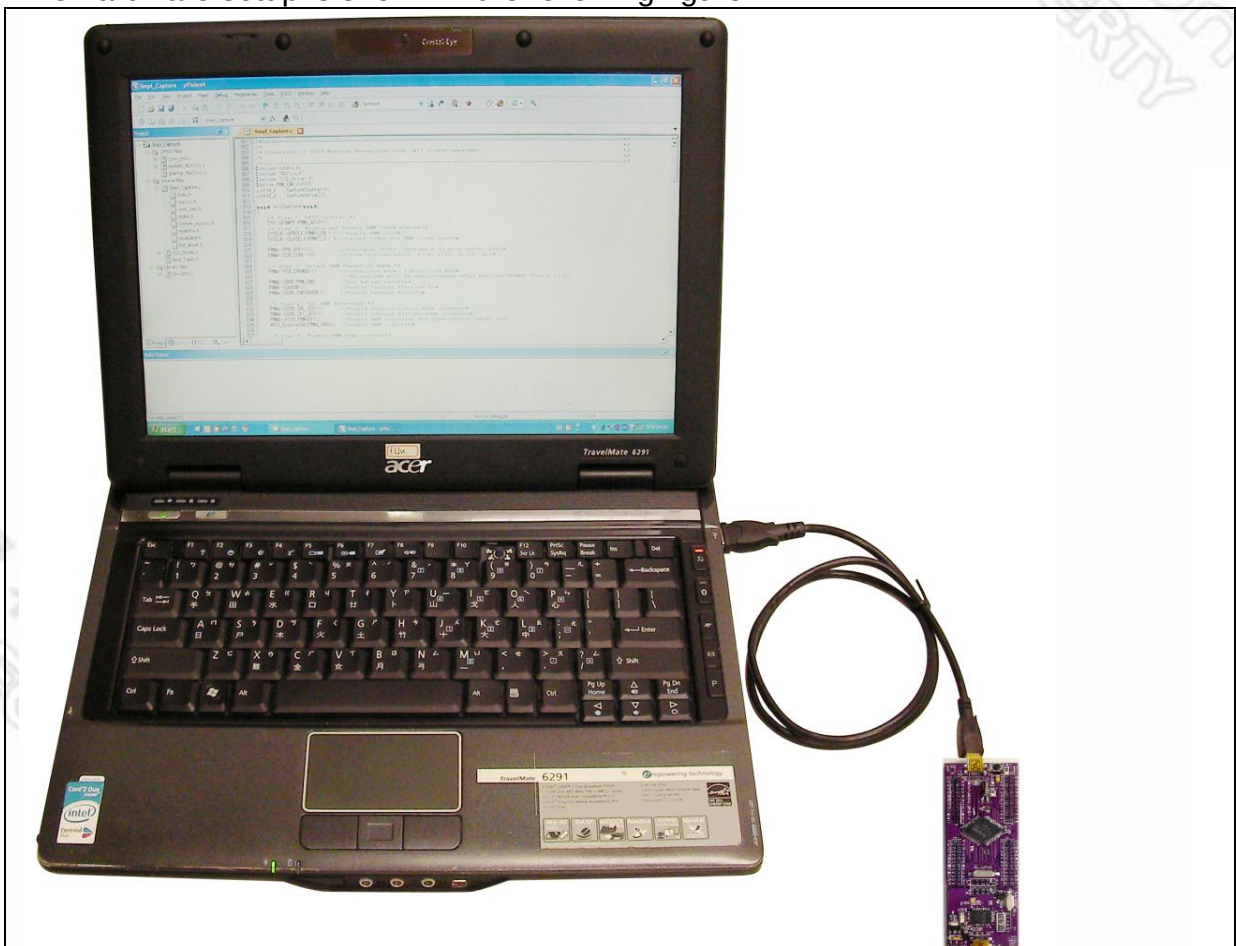
Figure 4-1 NuTiny- SDK-NUC220 Hardware Setup
