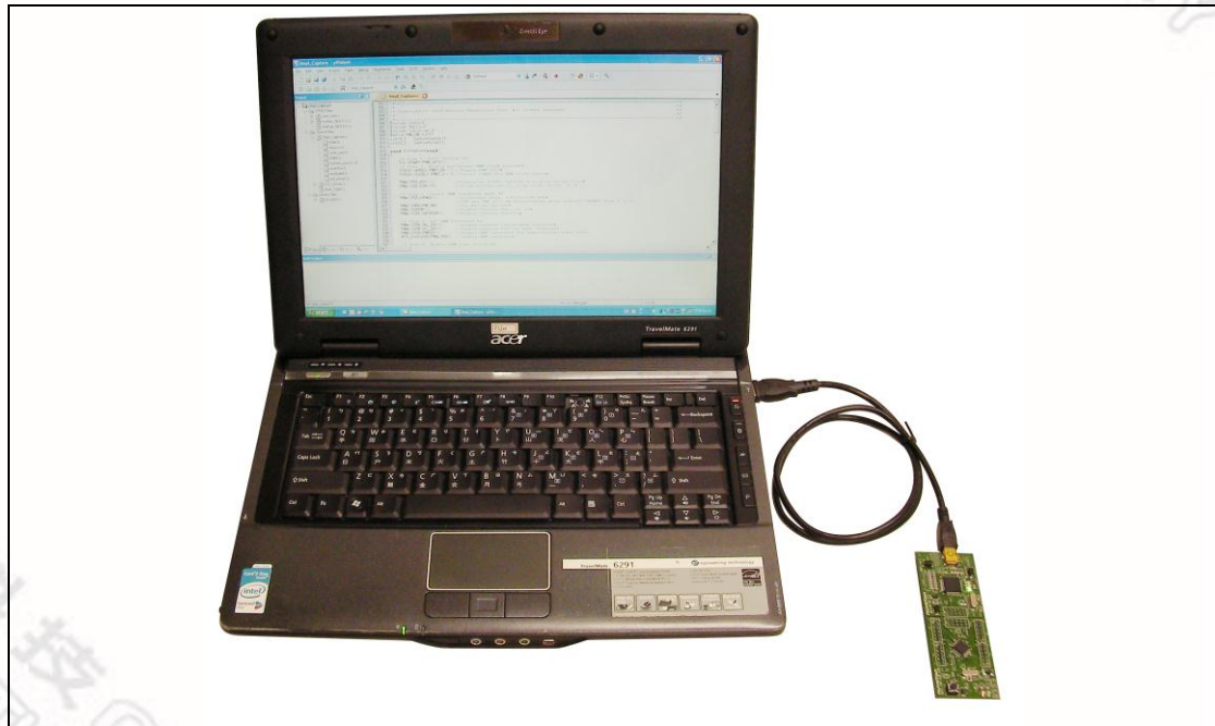
Figure 4-1 NuTiny-SDK-M058S Hardware Setup
