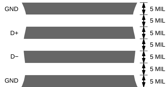
Figure 12. Typical Assignment of Signal Tracks
