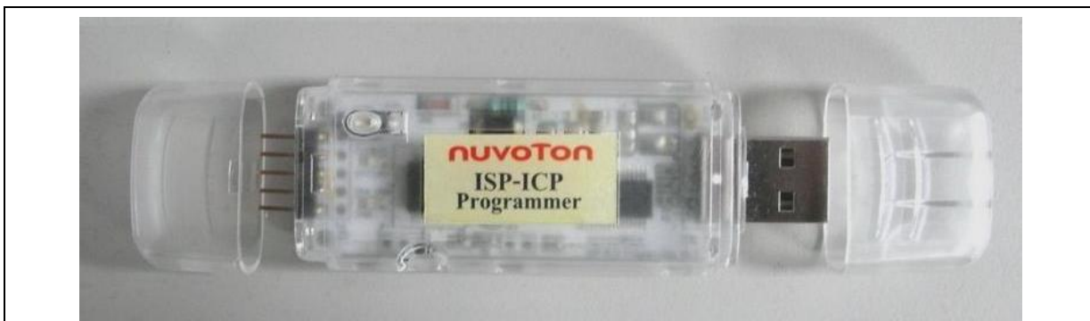
Figure 27–2 Nuvoton ISP-ICP Programmer
