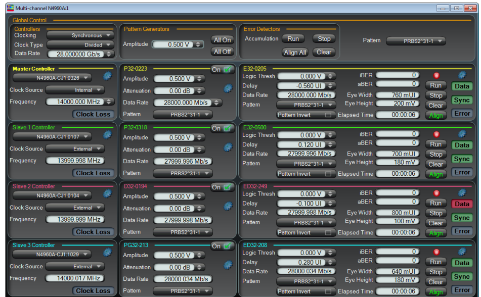
Figure 10. N4980A multi-channel BER measurement interface.
