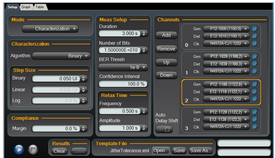
Figure 15. Jitter tolerance setup panel in N4980A.
