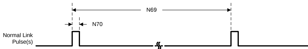
Figure 5-42. 10Base-TX Normal Link Pulse Timing
