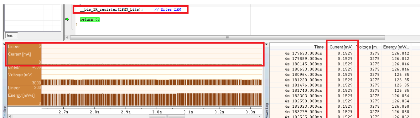
Figure 28. LPM3 Current When Executing Under Debug Control
