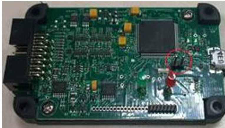
Figure 17. MSP-FET Rev 1.2 Jumper J5
