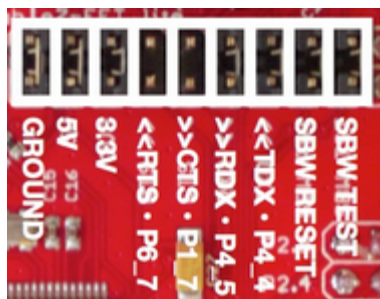
Figure 41. eZ-FET Lite Debug Connector
